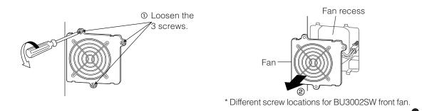
2. While pressing down on the tip of the fan connector ①, pull it toward you to disconnect it. ② The beep stops, and the error lamp turns OFF.
